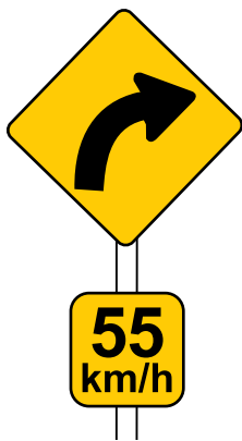
Road bends to right. 55 km/h maximum speed in good conditions.
